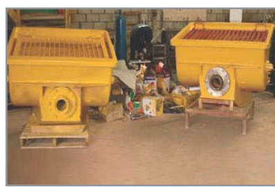
MSB905 HOPPER FOR STATIONARY AND TRUCK MOUNTED PUMPS
